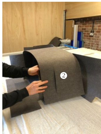
b). Lift outside panel (2) up and over inside panel (1) so they overlap and slots line
