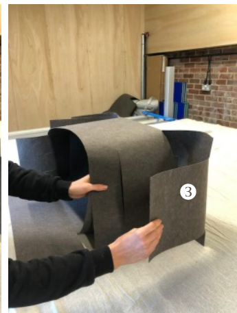
c). Thread post sleeve (3) through slots in (1) and (2)
