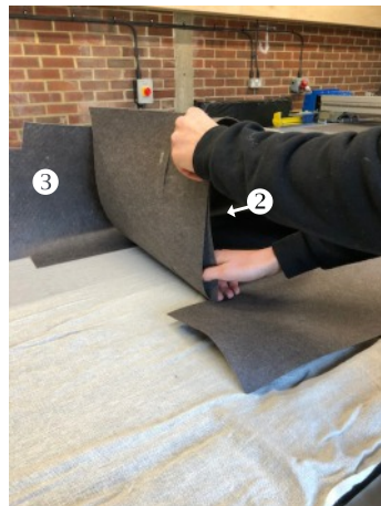
b). Lift outside panel (2) up and over inside panel (1) so they overlap and slots line
