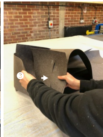
c). Thread post sleeve (3) through slots in (1) and (2)
